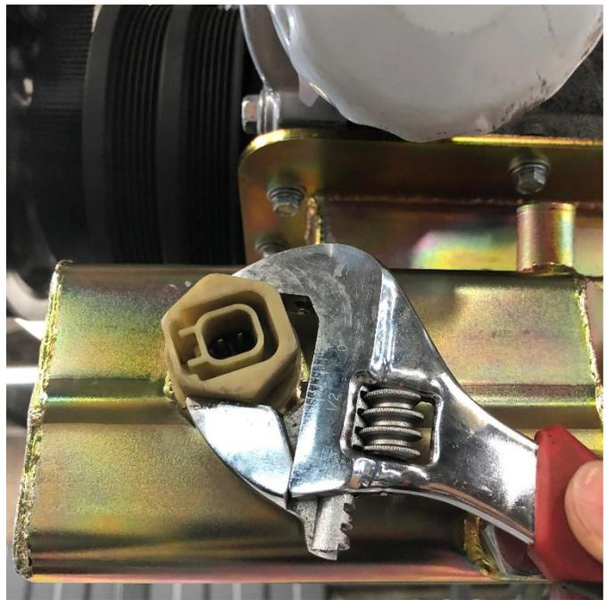
Remove the 4 temporary screws and install the oil pan tightening in an alternating pattern. Torque to 10 NM plus 45 degrees. The oil level sensor can then be reinstalled into the new pan.
