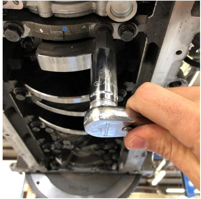
Use threadlocker on the front screw stud and reinstall the extension.
