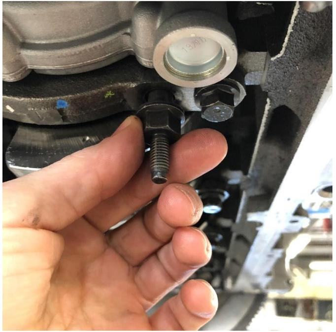
Remove the stud extension and cap screw from the rear of the block and reposition it into the front of the block. The cap screw at the front will replace the screw at the rear.
