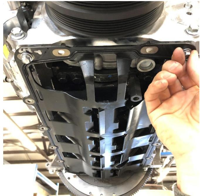
Apply RTV silicone to the 4 areas where the front and rear of the block meets the front cover and bellhousing areas. Lightly tighten 4 oil pan screws to hold the windage tray in place.
