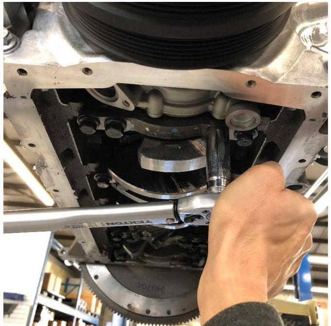
Torque both main cap screws to 65 NM.
