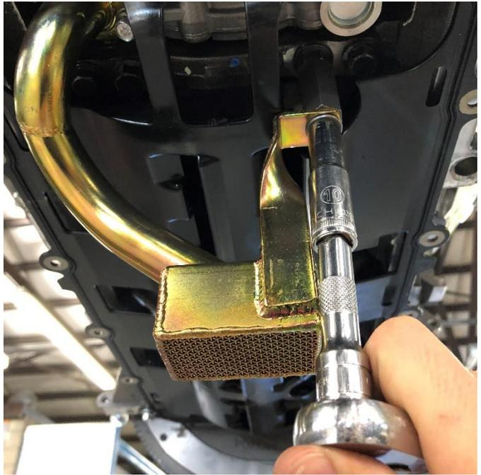
Using threadlocker, install the pick-up as shown and tighten all 3 bolts to 10 NM plus a 45 degree turn.
