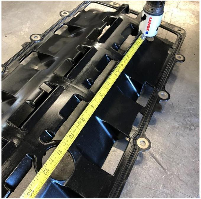
Remove the stock oil pan, oil pick-up, and windage tray. The locating pins on the factory Coyote windage tray will need to be removed. These pins aid in production assembly of the engine but are not required for this installation. To use a front sump pick-up, it's necessary to make a new hole in the windage tray 12 inches forward of the existing hole using a 1.25" hole saw or snips.
