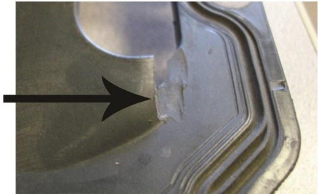
At the rear of the windage tray, 2 areas need to be ground for clearance to the new oil pan flange. The new oil pan and the tray should be checked so that they sit flat against one another.
